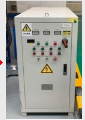
Induction heating instead hot air oven
