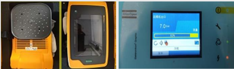
Compressor air pip leakage check by special device
