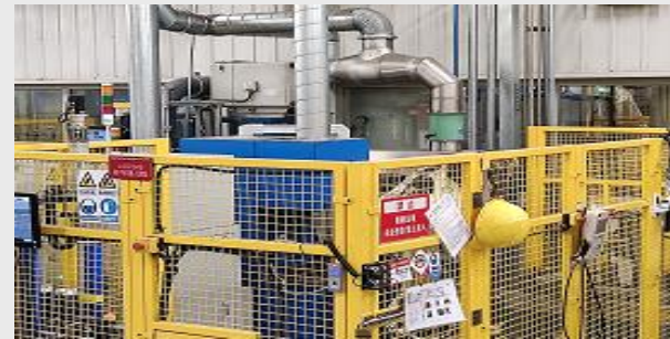
Exhaust fan stat and stop by compressors sensor
