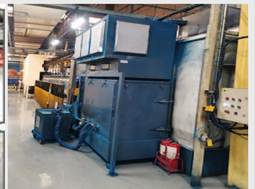
Painting oven, phosphating tunnel, powder painting booth start / stop automatic by sensor
