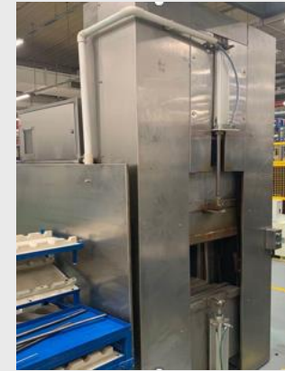
Induction heating instead hot air oven
